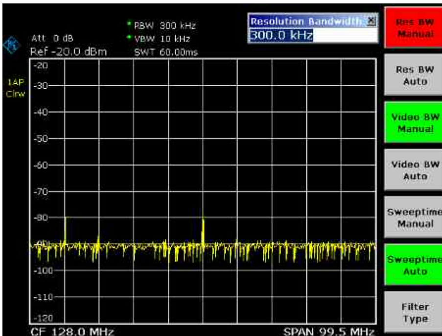
Fig. 2-13 Reference signal at a smaller resolution bandwidth
